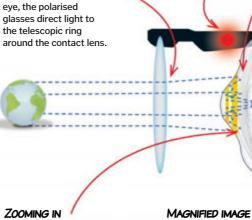
The mirrors bounce the light around the ring four times, magnifying the image by 2.8 times.
